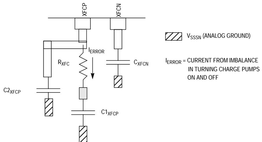
**Figure 4. Bypass Capacitor ( $C2_{XFCP}$ )
