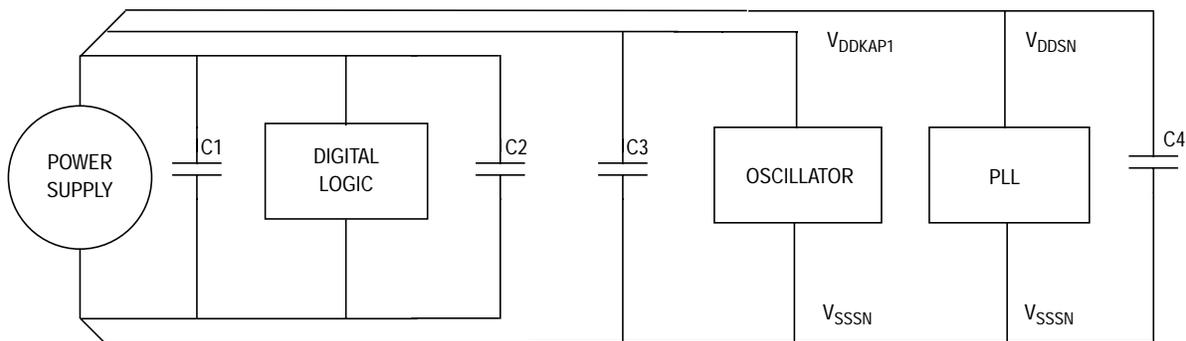
**Figure 6. Star Point Power Supply Connection**
