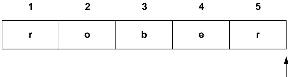
**Figure 4-4** shows the next write operation adds a new component to the file and moves the file pointer to the new end-of-file.
