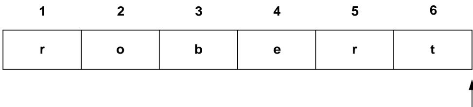
Reading up to the last byte of the file causes the next read operation to return an end-of-file status (see [Figure 4-3](#)). Trying to read past the end-of-file mark causes an error. To expand a file, simply write past the previous end of the file (see [Figure 4-4](#)).
