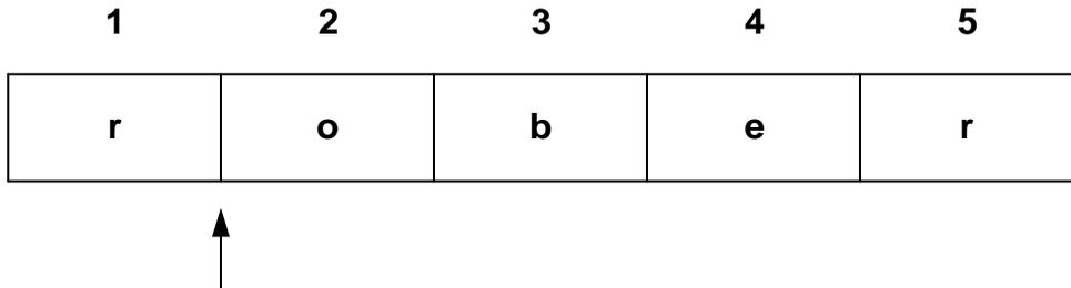
**Figure 4-3** shows the file pointer is pointing to the current end-of-file. Attempting another read operation causes an end-of-file error. Another write operation increases the size of the file.
