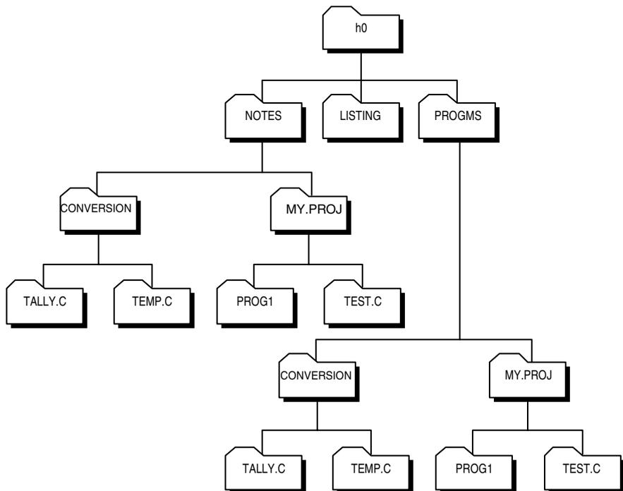
If the current working directory is the root directory of the disk, `dsave` creates a file that backups the entire disk, file by file. This is useful when you need to copy many files from different format disks or from a floppy disk or a hard disk.
