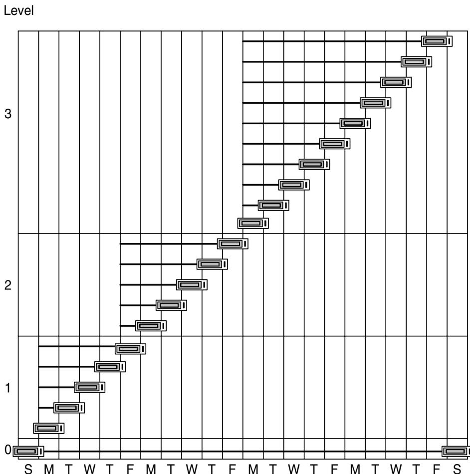
This strategy is designed for tape backups of larger systems. Tapes are used efficiently because a question as to how many tapes are needed never arises. This strategy also cuts down on person hours, tape mounting, and storage space used for tapes. It allows for enough redundancy to make restoring a full system fairly painless.
