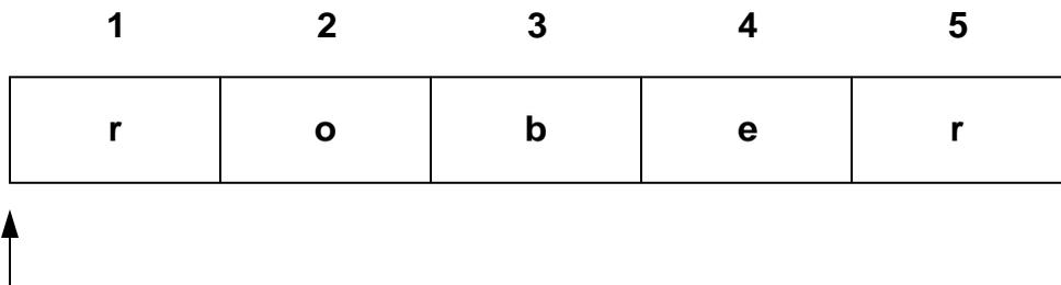
**Figure 4-2** shows after reading or writing the first component of a file, the file pointer points to the second component.
