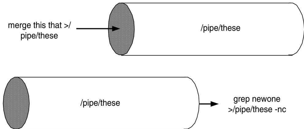
You can also create named pipes by writing to the named pipe from a program. Named pipes are similar to mass-storage files. Named pipes have attributes and owners. They may be deleted, copied, or listed using the same syntax one would use to delete, copy, or list a file. You may change the attributes of a named pipe just as you would change the attributes of a file.
