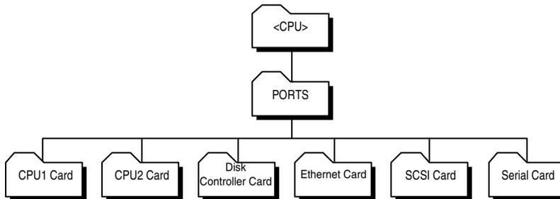
Generally, if you are going to use peripheral cards with a variety of CPU cards, you should locate them under the 68000 directories. Drivers and card ports specific to 68020 or CPU32 family processors would be located under their respective `<CPU>/PORTS` directory.
