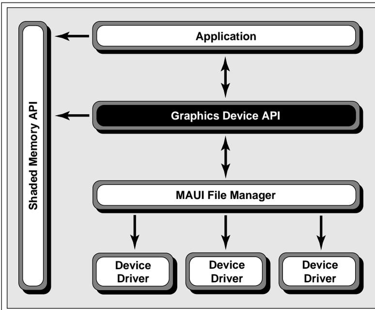
An application uses the Graphics Device API to perform hardware-dependent operations. These operations are transparent to the application. To make the Graphics Device API hardware-independent, the API must talk to the hardware through the MAUI file manager and graphics device drivers.
