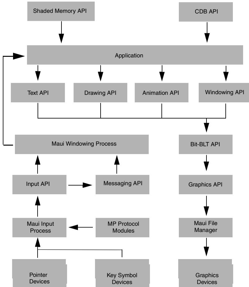
The Bit-BLT API can perform all block drawing and copy operations to drawmaps. However, if the CPU cannot access the pixel memory in the drawmap, the Bit-BLT function calls the driver to perform the operation.
