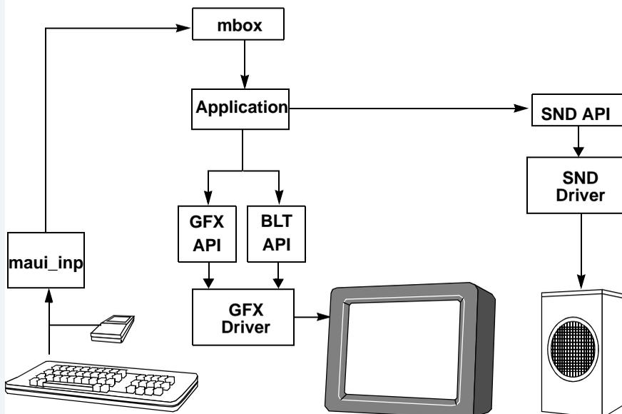
As shown in [Figure 1-1](#), the MAUI system comprises several components. At the heart of the MAUI system is a powerful set of APIs. These form the application interface to the MAUI system. For simplicity, the diagram shows most of the APIs in one block. However, this is actually a hierarchy of APIs. Each API has its own scope and objectives.
