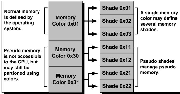
In this diagram, the operating system has defined one color of memory (color 0x01). The application is using this color to define shades 0x01, 0x02, and 0x03.
