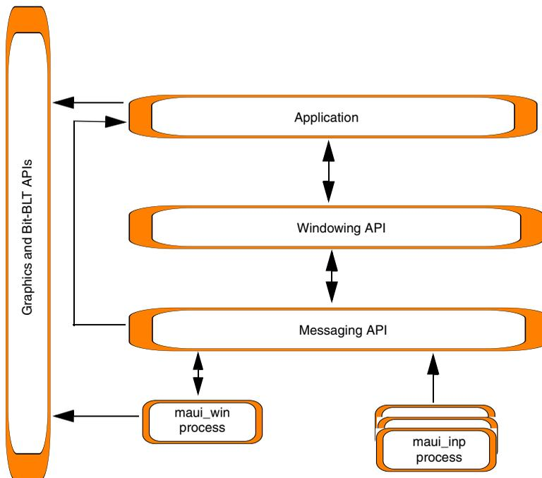
Before the Windowing API is used in an application, the Bit-BLT, Graphics, and Messaging APIs must be initialized. After the Windowing API is initialized (`win_init()`) set the action to take in the error handler by calling `win_set_error_action()`. The Windowing API is terminated when your application calls `win_term()`.
