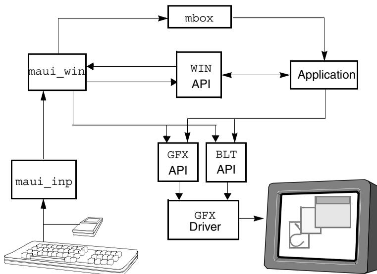
Applications call windowing functions, which are processed by the Windowing API. The Windowing API returns information to the application such as device and window IDs. Windowing commands are processed by the `maui_win` process.
