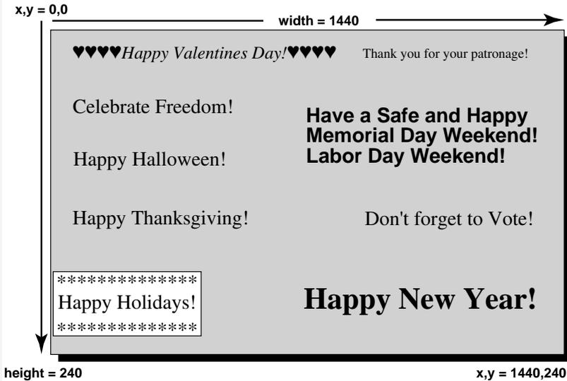
To display a portion of the image from the drawmap, identify the portion by the x,y coordinate of the top left corner of the partial image, and define the area in width and height of the partial. For example, the message Happy Holidays in the sample image is located at x,y coordinate 10,200, and occupies an area 350 pixels wide by 40 pixels high.
