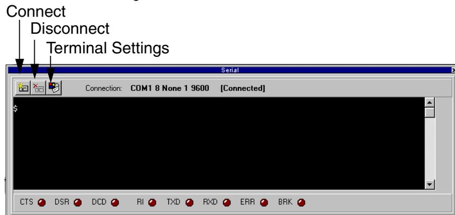
5. Once you have the Serial Console window open, click the **Connect** button in the upper left corner of the window. The Com Port Options dialog box appears.
