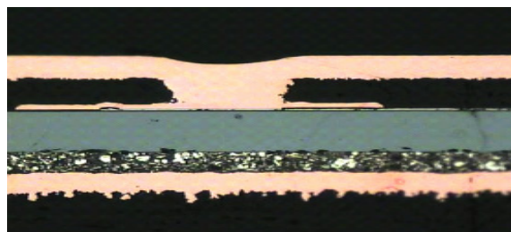
Figure 7 Cu-interconnection to embedded die
