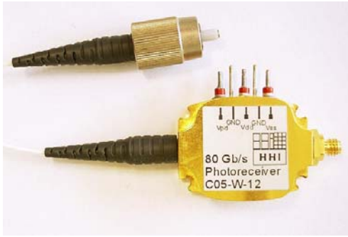
Figure 4: Components: Left A photograph of a pig-tailed OEIC 80 Gbit/s receiver module with 1mm RF output Right: 43 Gbit/s MZI-Modulator module with GPPO RF connector
